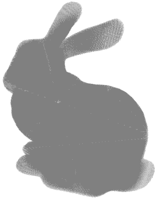
Figure 12: Plot of the peridynamic material points of the bunny. The size of the scattered bunny is [-0.04, 0.04] \text{ m} \times [-0.03, 0.04] \text{ m} \times [-0.06, 0] \text{ m} .
